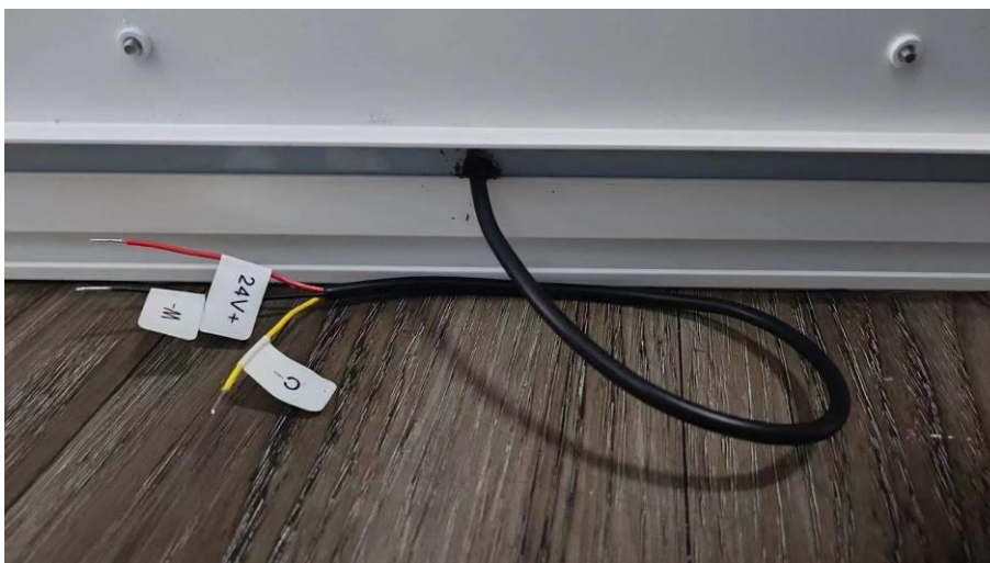
Wire entry view of CS-LBPR series
