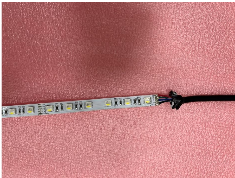
LEDs view of CS-LPPF-RGBW-120-24
